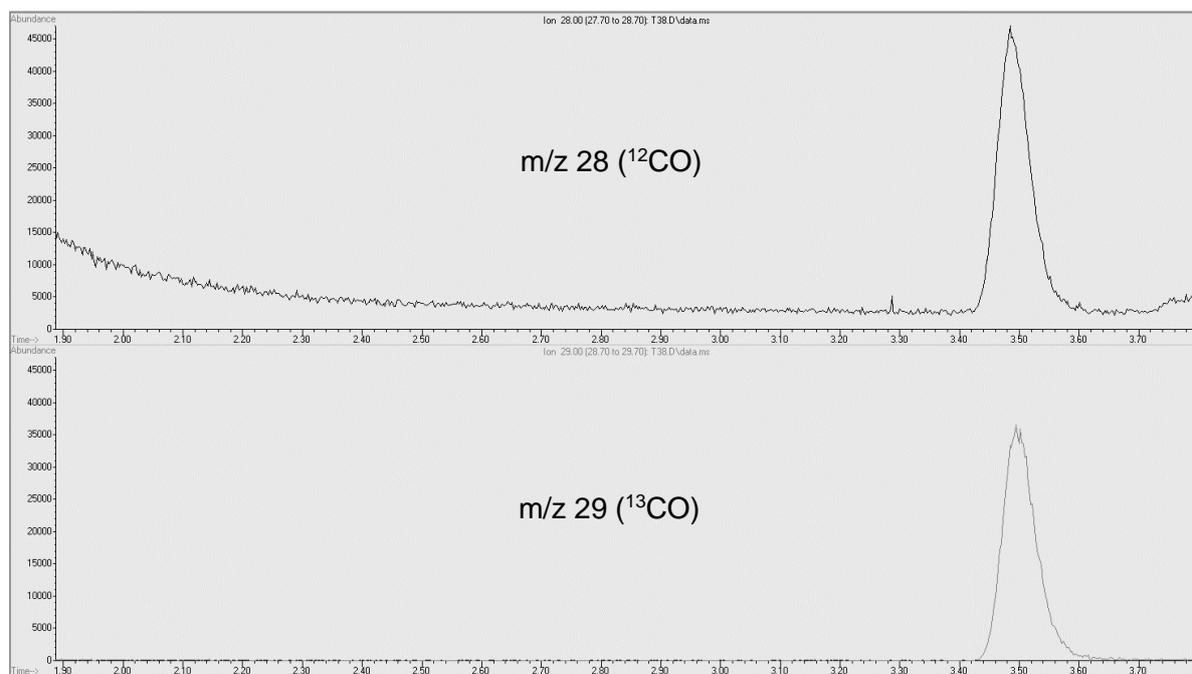
**Figure 3.1:** Extracted ion chromatograms for *m/z* ratios 28 (upper) and 29 (lower), corresponding to CO and  $^{13}\text{CO}$  respectively, for selectivity tests.
